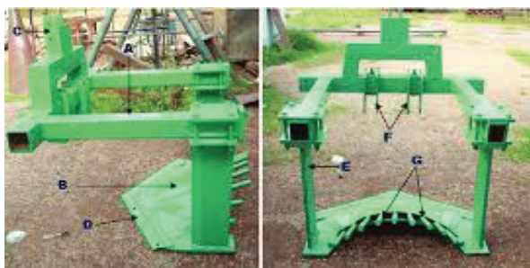
A – Beave to which digging unit is attached C – Top link hitching point E – Vertical support G – Slatted rods for shaking off soil
